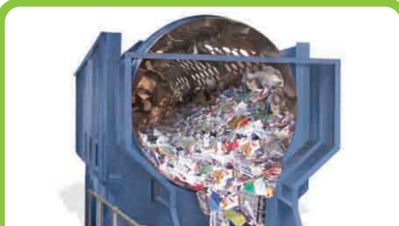
The rotating 'trommel' filters out any remaining small items, leaving paper, cardboard and orange sacks behind.
