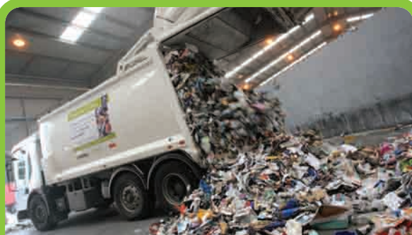
Recyclables are tipped into a tipping bay and inspected for quality purposes.
